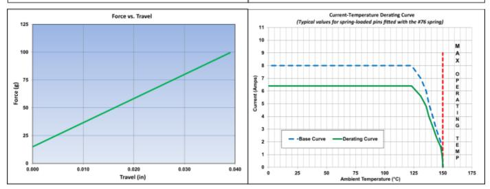
The stroke, force and current rating values are measured using spring pins with an internal construction per the design specification.
